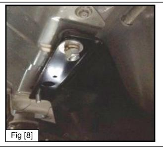
**Step 10.** Torque the 1/2" hardware to 70ft-lbs and the 7/16" hardware to 65ft-lbs. Reinstall the impact bar and bumper by following these steps in reverse starting at Step 6. Torque the impact bar nuts to 33ft-lbs. Using an air saw, dremmel, or utility knife, trim the bumper tabs shown in Figure [9] or tuck upwards out of the way. See Figure [9].
