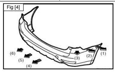
**Step 6.** Remove the nuts securing the impact bar to the vehicle. After all nuts are removed, raise the whole impact bar a little to remove it from the vehicle body.
