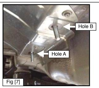
**Step 9.** Raise the hitch into position on the fished bolt hardware being careful not to push the hardware back into the frame rail. Attach (2) 1/2" flat washers, (1) 1/2" lock washer, and (1) 1/2"-13 hex nut to the 1/2" hardware and hand tighten. Attach (2) 7/16" flat washers, (1) 7/16" lock washer, and (1) 7/16"-14 hex nut to the 7/16" hardware and hand tighten. See Figure [8].
